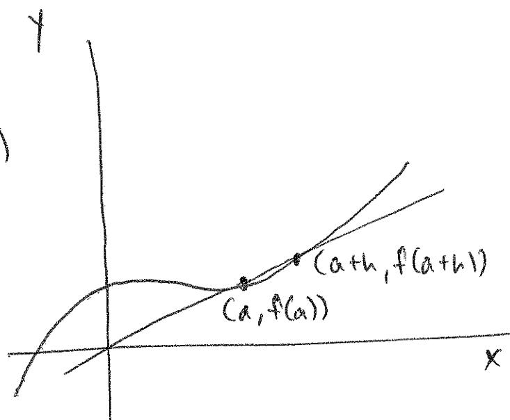
the quantity inside the limit. As  $h$  approaches zero, the two points both approach  $(a, f(a))$ , so that the line in the picture approaches the tangent line to the graph at  $(a, f(a))$ . Thus, the derivative is the limit of this slope, i.e. the slope of the tangent line.
