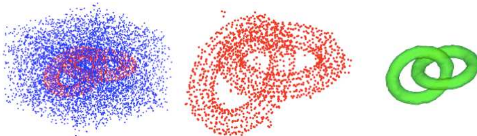
Figure 2: a) Data with 500% noise, b) Data filtering by tensor voting, and c) Reconstructed surface.
