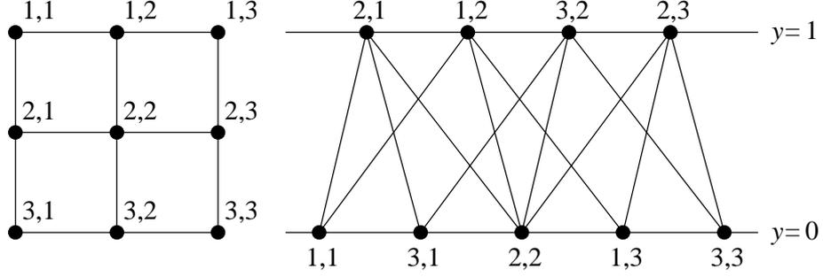
**Fig. 2:** Mesh  $\mathcal{M}(3, 3)$  and its optimal bipartite drawing
