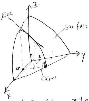
The surface is Z = f(x,y). The curve on the Surface is The intersection of Z = f(x,y)Surface is The intersection of Z = f(x,y)and X = Q. The line is the line tangent to the intersection of Z = f(x,y)
