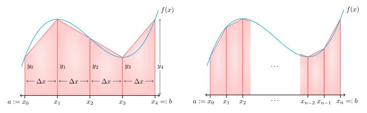
Assume the length of each subinterval is  $\Delta x = \frac{b-a}{n}$ . Then the area of the trapezium that lies above the *x*-axis in the *i*<sup>th</sup> subinterval is  $T_i = \frac{\delta x}{2} (y_{i-1} + y_i)$  where  $y_{i-1} = f(x_{i-1})$  and  $y_i = f(x_i)$ . Then the area of the under the curve and above the *x*-axis is approximated by the sum of the trapeziums:
