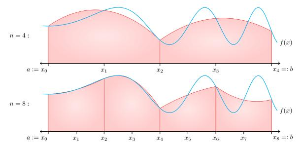
So how do we compute the area under each parabola  $y = Ax^2 + Bx + C$ ? By translating we can assume that the centre point of our parabola is at  $x_i = 0$
