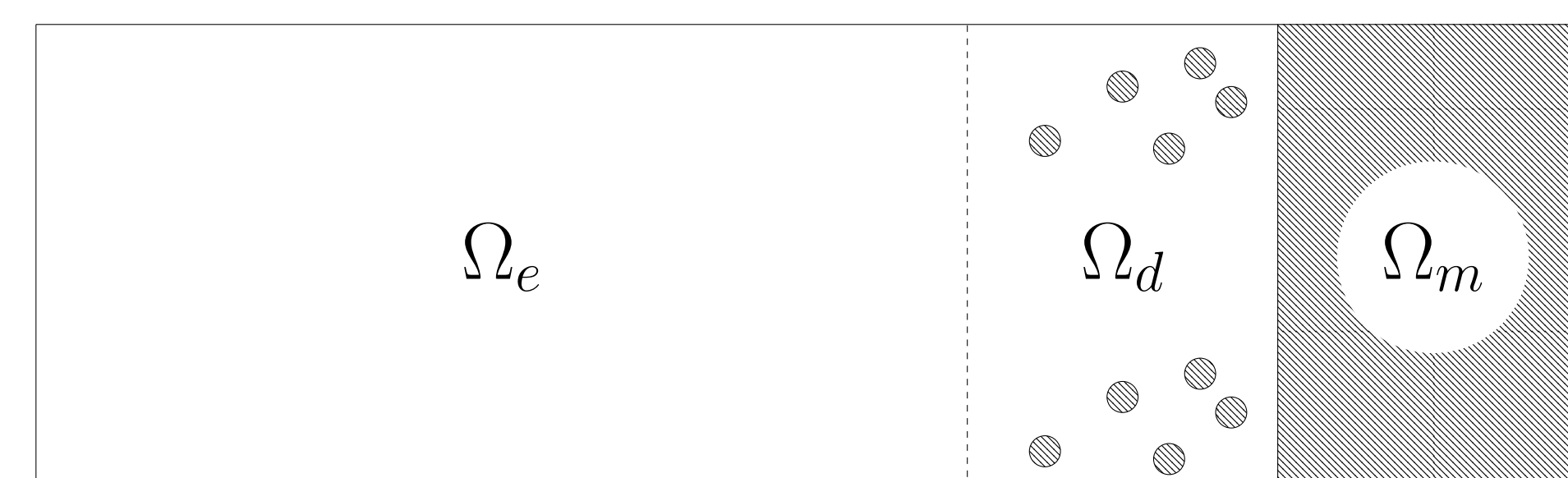
Figure 3: The 1D model will involve three regions. The electrolyte solution \Omega_e , the bulk metal \Omega_m , and the interaction region \Omega_d
