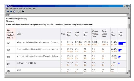
The following figure shows a summary of all the functions executed during the profile collection time. The **Manual Comparison Selection** of **max Time Aggregate** means that data is considered from all the labs for all functions to determine which lab spent the maximum time on each function. Next to each function's name is the lab that took the longest time to execute that function. The other columns list the data from that lab.
