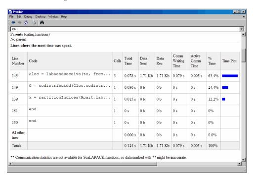
The code that is displayed in the report is taken from the client. If the code has changed on the client since the parallel job ran on the labs, or if the labs are running a different version of the functions, the display might not accurately reflect what actually executed.
